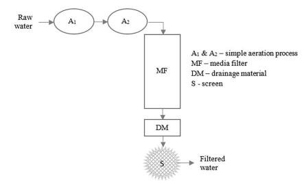
Figure 5. Schematic diagram of the water path
