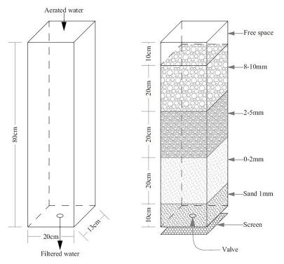
Figure 3. Physical model for experiment: (a) Model dimensions, (b) Layers of material in the model
