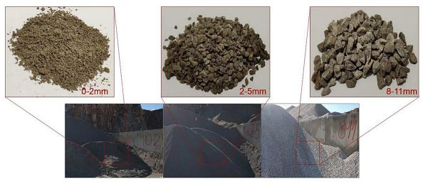
Figure 2. Limestone grain sizes used for filter media
