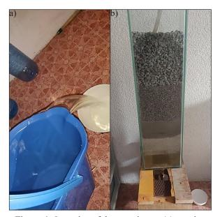
Figure 4. Operation of the experiment: (a) aeration of raw water, (b) filtration of aerated water
